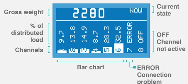
The TLM8 displays graphically the load cells response signal in mV for each active channel.
