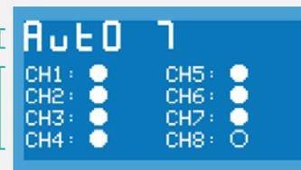
**Active Channels:** there is a connection with the load cell.
