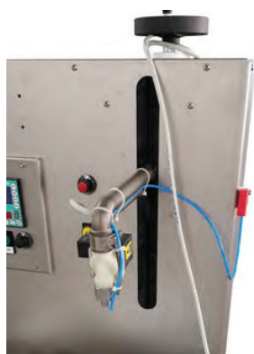
9037 Manual valve for nitrogen injection
