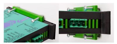
Tighten the four screws up to lock the instrument.
