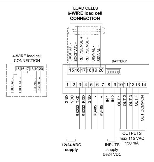
4 outputs: controlled by setpoint values or by remote device via protocol.
