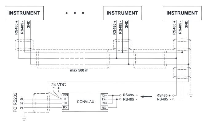
If the RS485 network exceeds 100 metres in length or baud-rate over 9600 are used, two terminating resistors are needed at the ends of the network: close the two jumpers indicated in the picture on the furthest instruments. Should there be different instruments or converters, refer to the specific manuals to determine whether it is necessary to connect the above-mentioned resistors.
