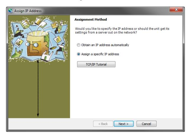
Select Assign a specific IP address, enter the desired values and click on Assign; wait for the procedure to complete (no need to restart the instrument).
