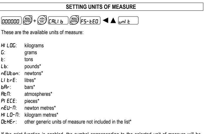
If the print function is enabled, the symbol corresponding to the selected unit of measure will be printed after the measured value.
