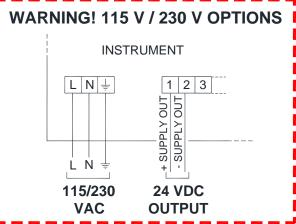
**WARNING:** connect power supply specified on the plate found on the back of the instrument. In 115 V and 230 V versions, terminals "+ SUPPLY" and "– SUPPLY" generate continuous voltage at 24 VDC only to be used as power supply for instrument inputs.
