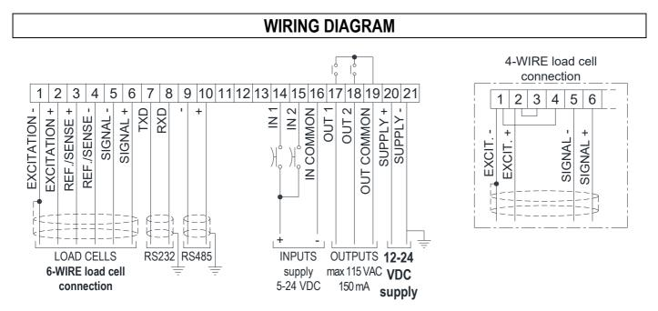
2 outputs: controlled by setpoint values or by remote device via protocol.
