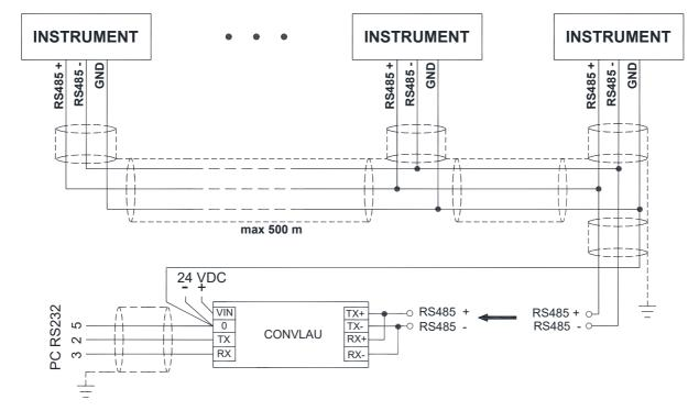
If the RS485 network exceeds 100 metres in length or baud-rate over 9600 are used, two terminating resistors are needed at the ends of the network. Two 120 ohm resistors must be connected between the "+" and "-" terminals of the line, on the terminal strip of the furthest instruments. Should there be different instruments or converters, refer to the specific manuals to determine whether it is necessary to connect the above-mentioned resistors.
