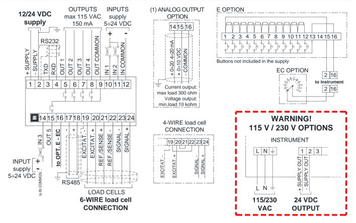
**5 outputs**: controlled by setpoint values or by remote device via protocol.
